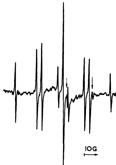
E.s.r. spectrum of the radical Me 3 SnCH 2 \dot{C}H_2 obtained by the photolysis of di- t -butyl peroxide in the presence of trimethylisobutyltin in ethylene at -70^\circ C [reactions (8) and (9)]. The arrows indicate two of the three lines of the spectrum of the radical Me 2 Bu 1 SnCH 2 ; the third line is obscured by the spectrum of the 2-trimethylstannylethyl radical
